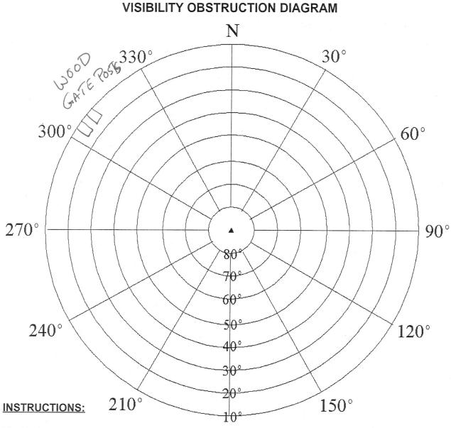
Identify obstructions by azimuth (magnetic) and elevation angle (above horizon) as seen from station mark. Indicate distance and direction to nearby structures and reflective surfaces (potential multipath sources).
