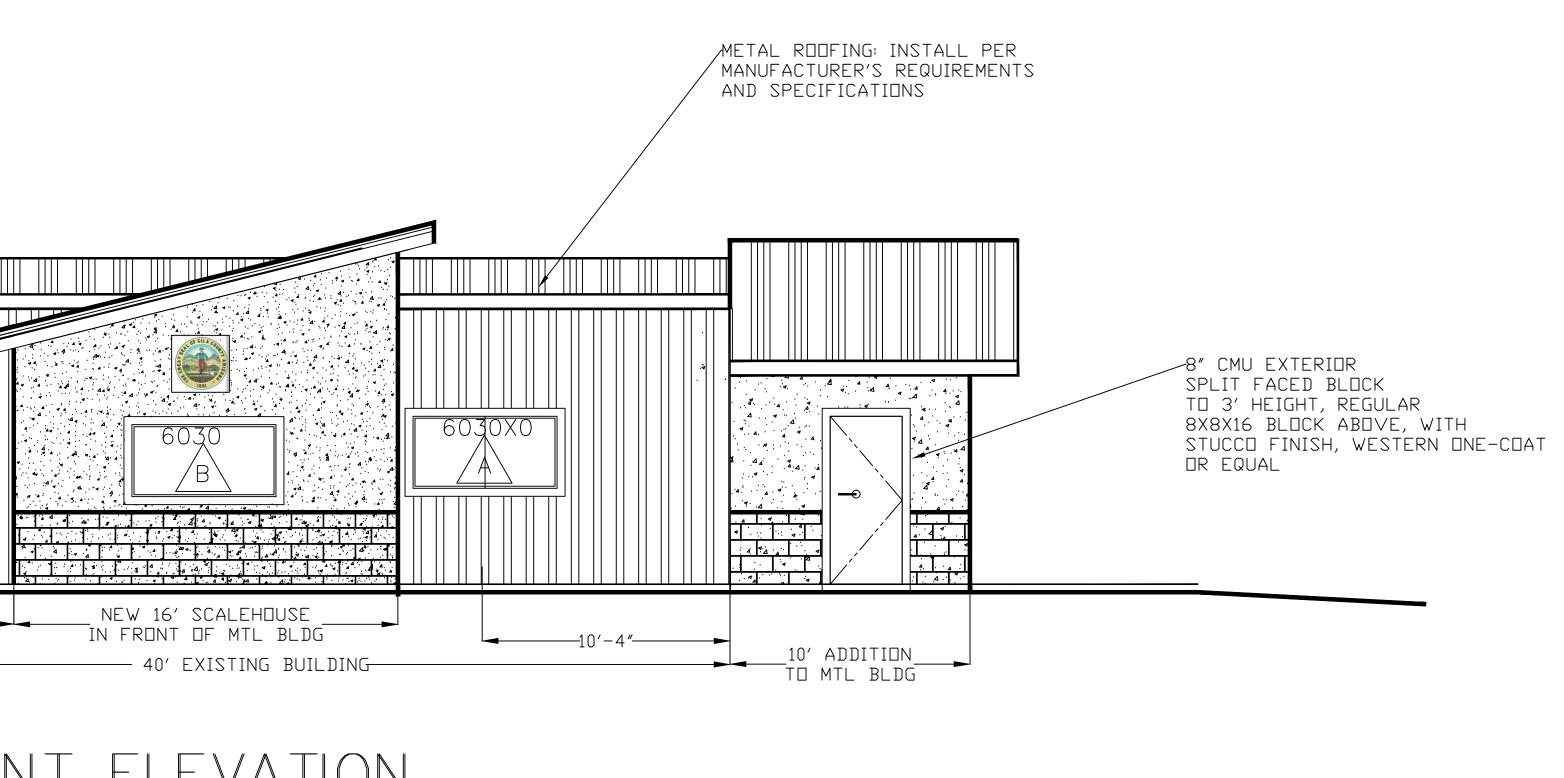
FRONT ELEVATION 4" CONC. SLAB OVER 4" ABC, OVER COMPACTED FILL . SEE SOILS REPORT. SCALE: 1/4" = 1' - 0"SLOPE SLAB AWAY FROM BLDG.
