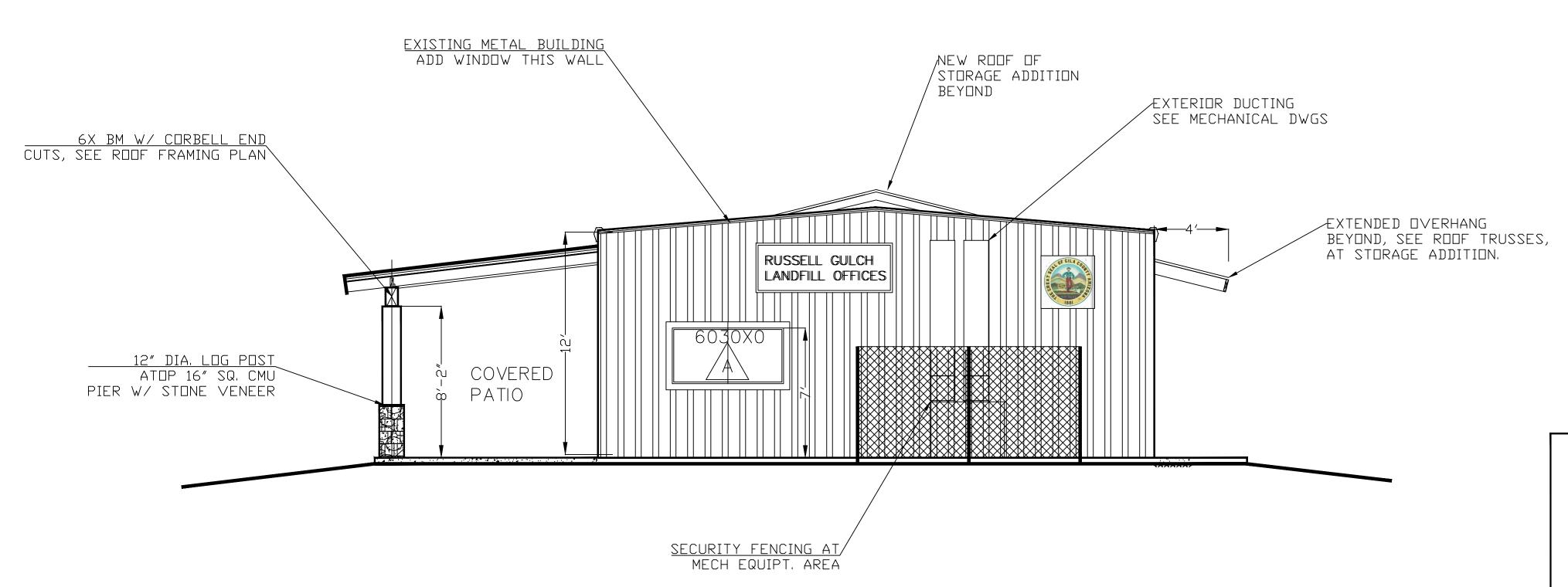
8" CMU EXTERIOR WALLS TO 10' HT. SPLIT FACED BLOCK TO 3' HT.
